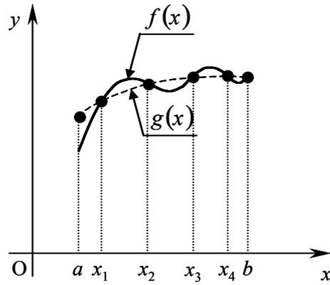
Figure 1: Equality of two functions:  $f(x) = g(x)$  from the collocation method point of view
