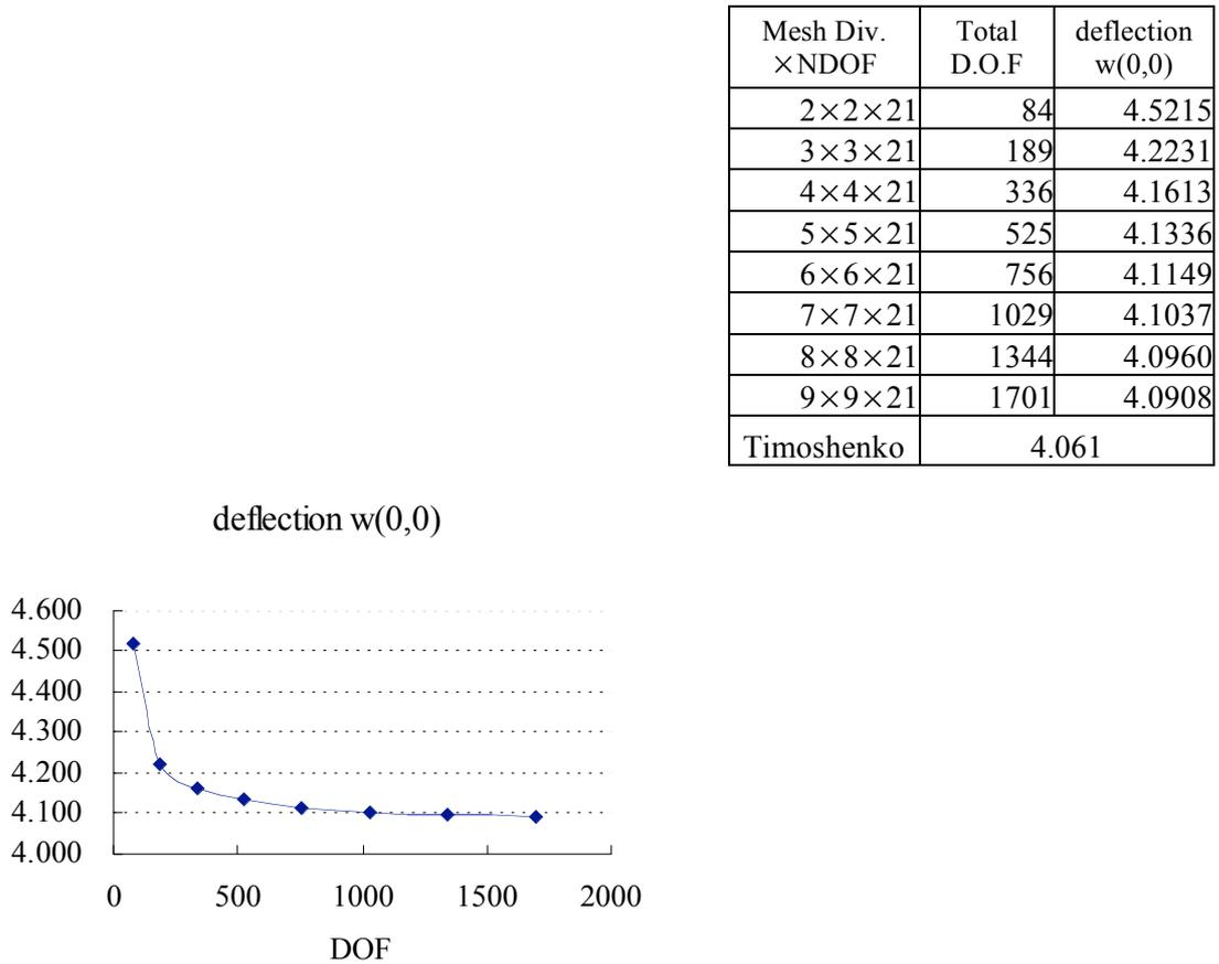
Figure 8: Bending analysis of a simply supported square plate displacement function used: 5th order polynomials of  $(x, y)$  (NDOF=21)
