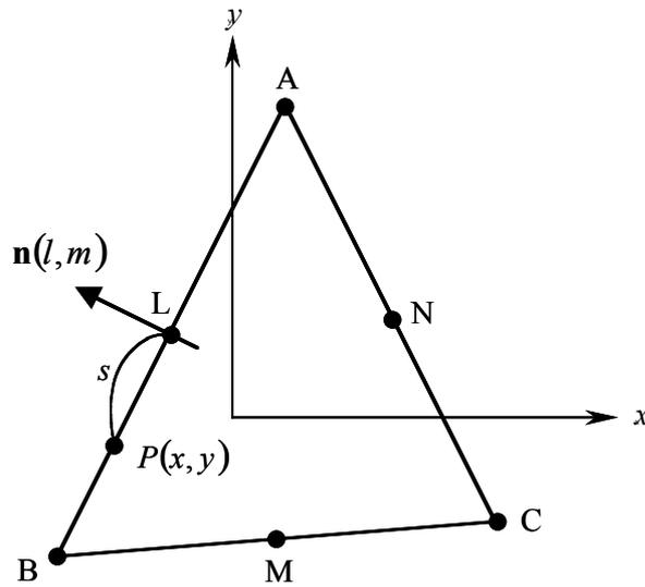
Figure 2: Development of a nodeless finite element
