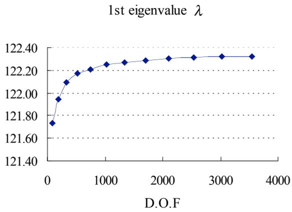
Figure 9: 1st eigenvalue analysis of a simply supported square plate displacement function used: 5th order polynomials of  $(x, y)$  (NDOF=21)
