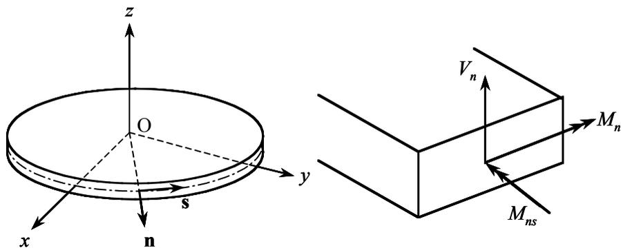
Figure 3: Coordinates and components of the traction vector for the plate bending problem
